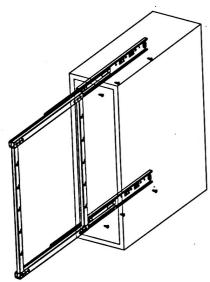
Drill 4 x Dia.2.5 holes one the door as below, fix the L shape fixing plate by screws.
