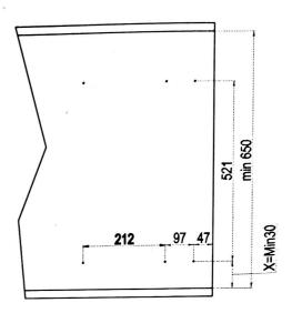
2 Install the frame to the cabinet, fix by 6 pcs screws.
