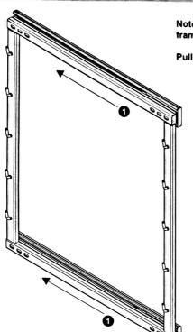
Note: Wirework may be supplied already placed on runners. For ease of fitting, remove frame with following guidance before constructing cabinet.
