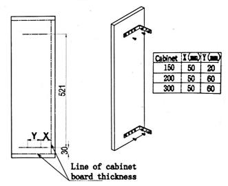
Connect between the door and the frame, make adjustment for the door as below:
